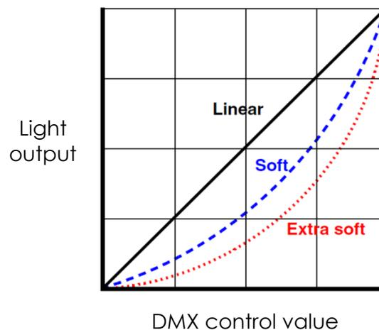
**Figure 3. Dimming curves**
