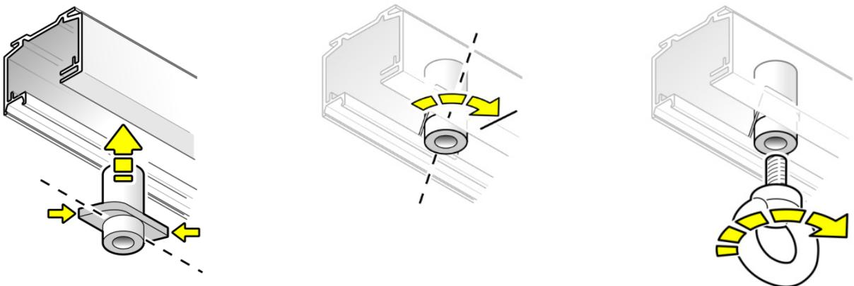
**Figure 8. Installing a retaining collar and safety cable**
