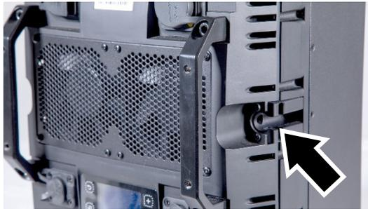
**Figure 5. Mechanical connector channel**
