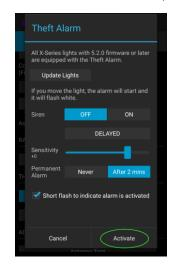
First make sure your Radio Pin is different from 0000. See chapter 7.1 how to change it. Then press the "ON" button. Press "Activate". All targeted lights will flash shortly to indicate that they are now armed.
