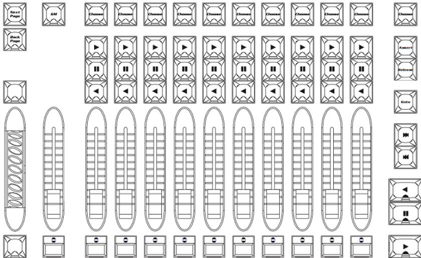
Figure 31.3. Playback section of the Hog 4 front panel
