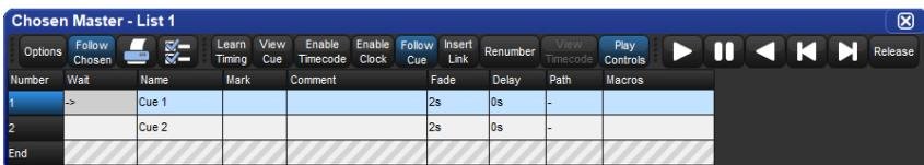
The controls are, from left to right, the Go, Halt/Back, Skip Back, Skip Forward, and Release buttons. These controls function independently from their front panel equivalents and always execute based on how they are labeled.
